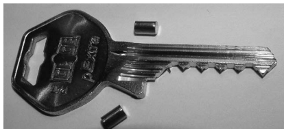
Figure 7-7 A typical bump key for a door.
