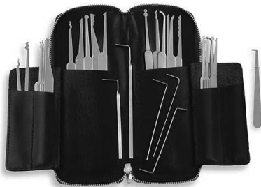
Figure 7-4 This lock-pick set is bulkier but contains everything you would need.
